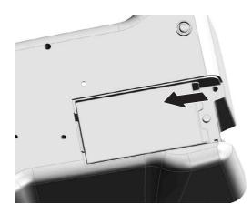
**8.** Push in the battery so that the contacts of the instrument can be plugged into the socket of the battery.
